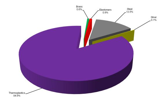
The materials used in the product range and the corresponding weight are disposed below, in *table 1*. The information about the constituent materials is referring to model CSW-CK2F45-10000000-3VF.
