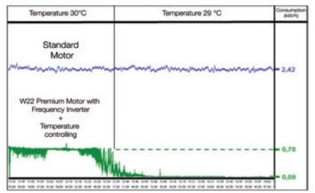
Measurements carried out to compare energy consumptions between Standard motors (standard efficiency) and W22 Premium (high-efficiency) motors with CFW701 HVAC Frequency Inverters.
