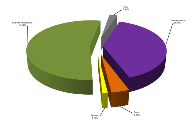
The materials used in the product range and the corresponding weight are disposed below, in *table 1*. The information about the constituent materials is referring to model PFW03-M24.
