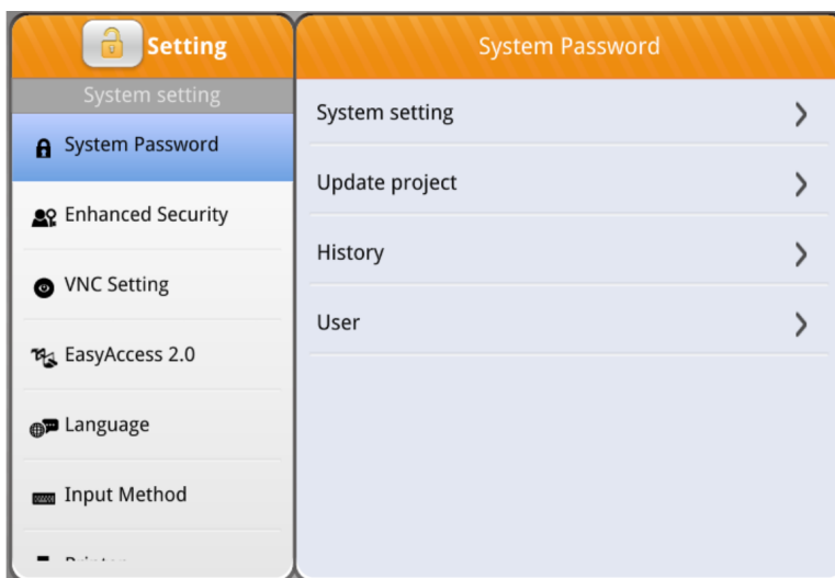
Figure 5.7: System password configuration for remote access.
