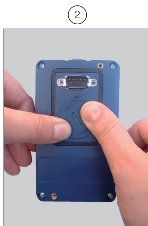
Press the cover and rotate it counterclockwise
