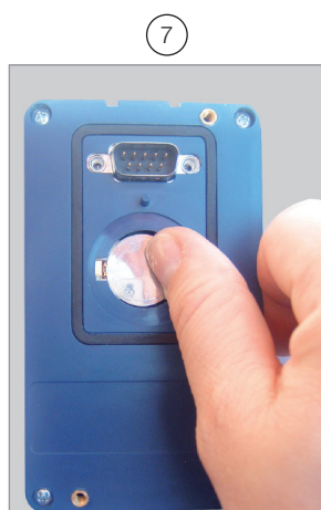
Press the battery for its insertion
