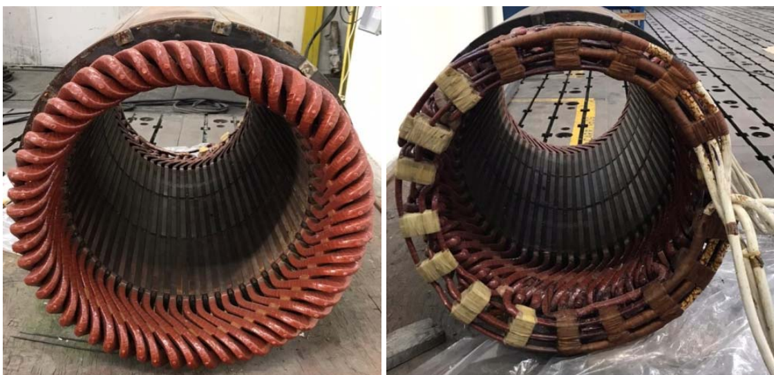
Figure 11: Sample of high voltage stator (Source: WEG)
