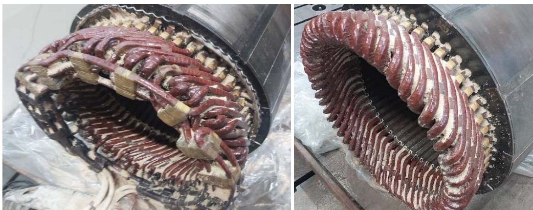
Figure 13: Sample contaminated with fine moist sawdust (Source: WEG)
