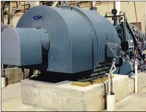
Synchronous motor with PMDP™ enclosure driving a refiner.
