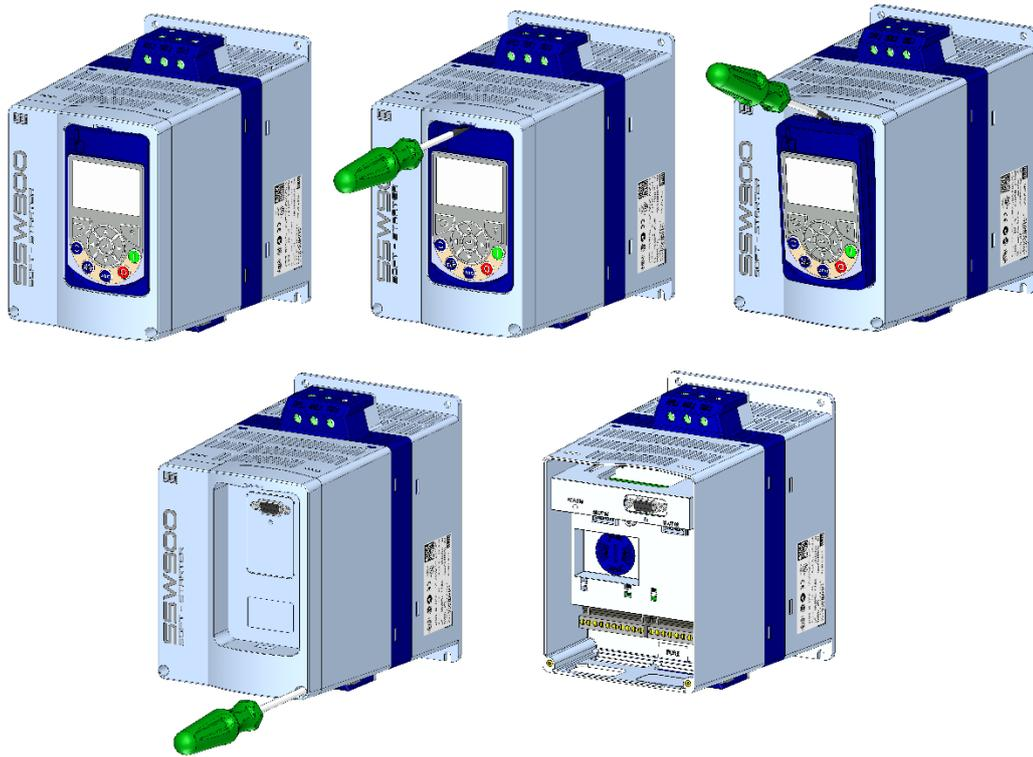
Figure 3.15: Removal of the HMI and front cover
