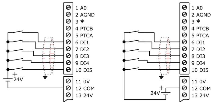
Figure 3.19: Wiring diagram of the digital inputs using external power supply
