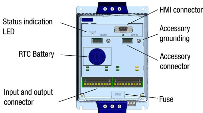
Figure 2.2: Access to the control of the SSW900
