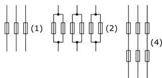
Table 3.13: Recommended Weg aR fuses delta inside connection with the fuses outside of the delta
