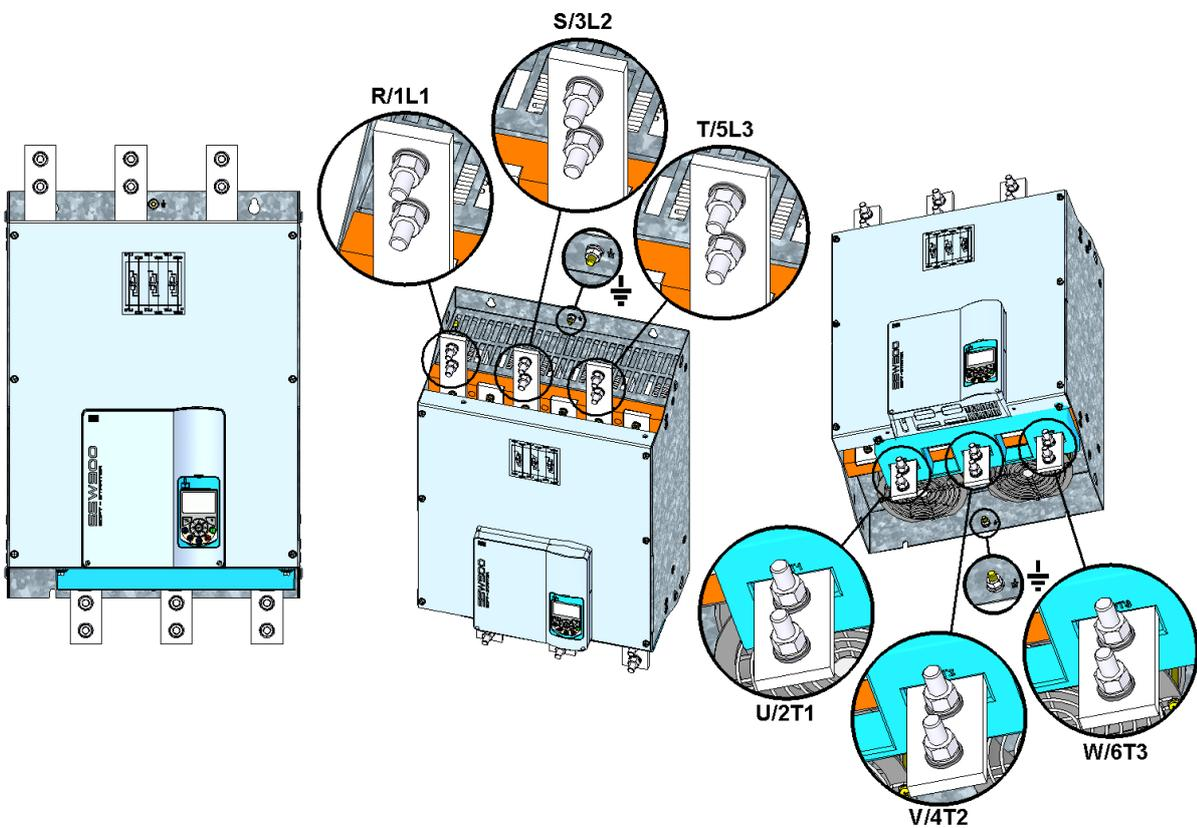
Figure 3.9: Power and grounding terminals, frame F
