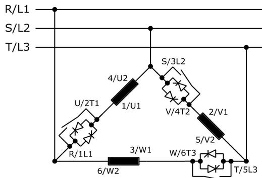
Figure 3.12: SSW900 inside delta motor connection with motor in delta
