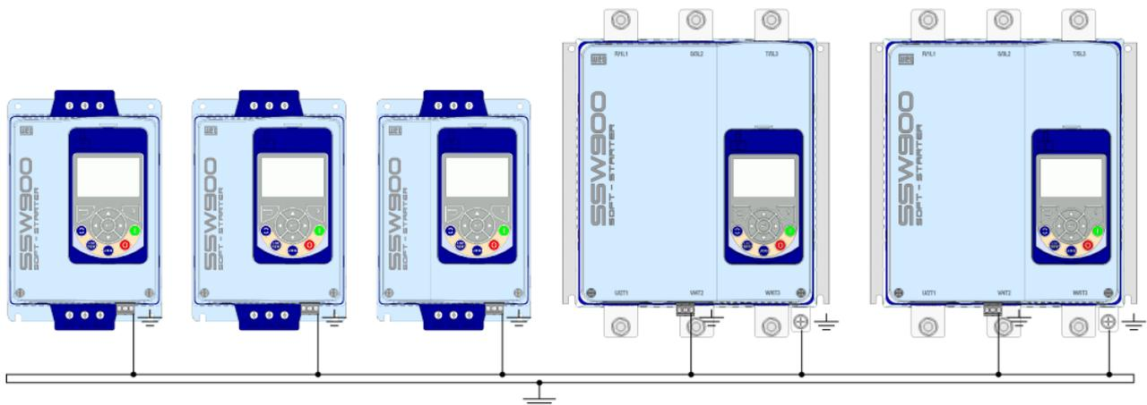
Figure 3.14: Grounding connections for more than one SSW900
