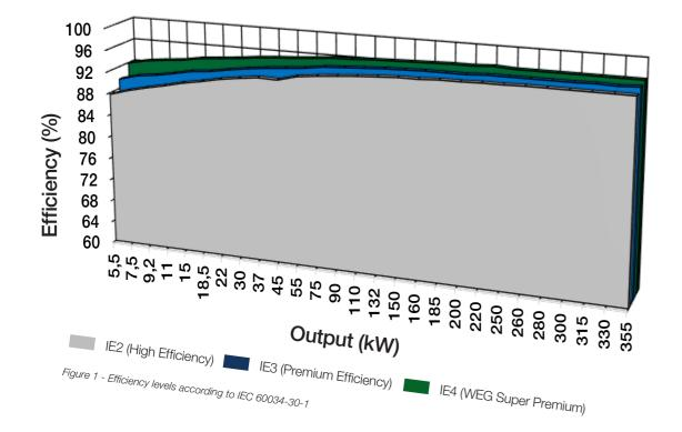
Figure 1 above provides a comparison between the efficiency levels for 4-pole, IE2 and IE3 machines with the W22 Super Premium IE4 design, respecting the levels defined in the IEC standard 60034-30-1:2014.
