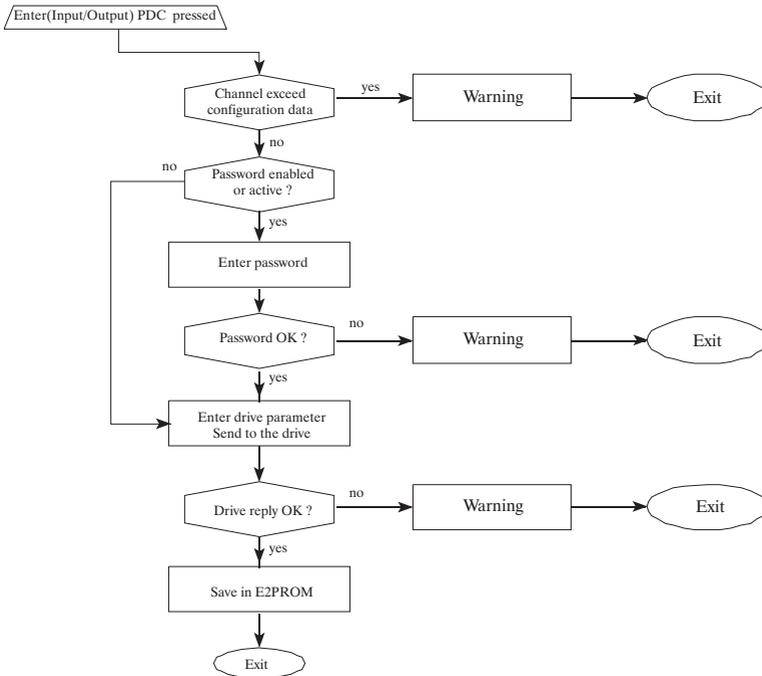
The validity of the specified Drive parameter is checked by the Drive. If the Drive responds with an error code, the following message is shown on the keypad Display:
