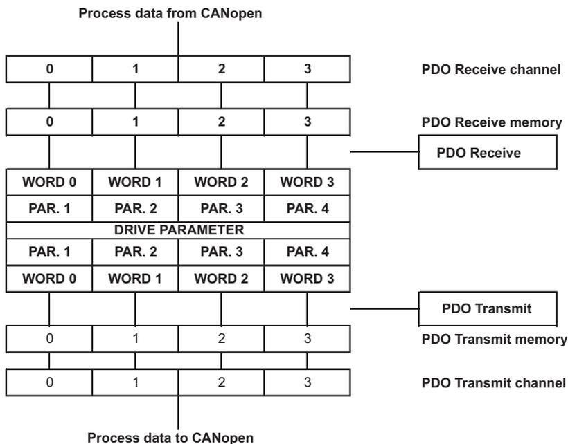
The "PDO Transmit" communication object (input data for the Master) defines the drive parameter assigned to the Process Data Object Words.
