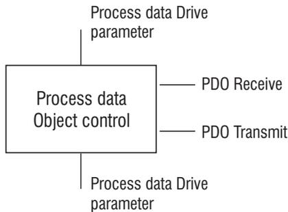
The Slave parameters are cyclically read by the Master by assigning the drive parameters to the "PDO transmit" communication object.
