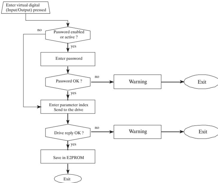
The validity of the specified Drive parameter is checked by the Drive.
