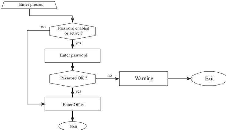
The Offset default value is 0; the entered value is not stored in a non-volatile memory and therefore it remains active only until the power supply is disabled; the Offset is however maintained active even after leaving the SBI main menu.
