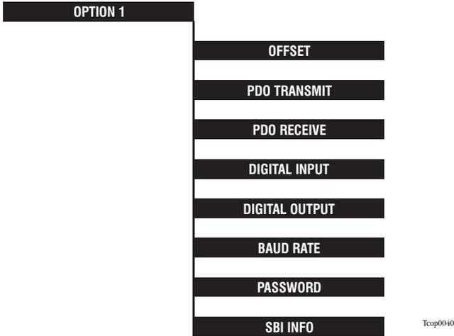
Move among the Menus by pressing the Cursor-Up/ Cursor-Down keys and use the Enter key to enter the currently displayed Menu. By pressing the Cancel key in any displayed menu, the "OPTION1" Menu appears and the keypad control returns to the drive.
