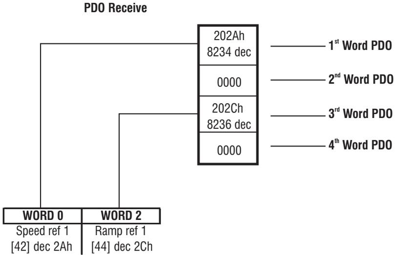
**NOTE:** The values 0000 mean that the Word is not assigned to any drive parameter.
