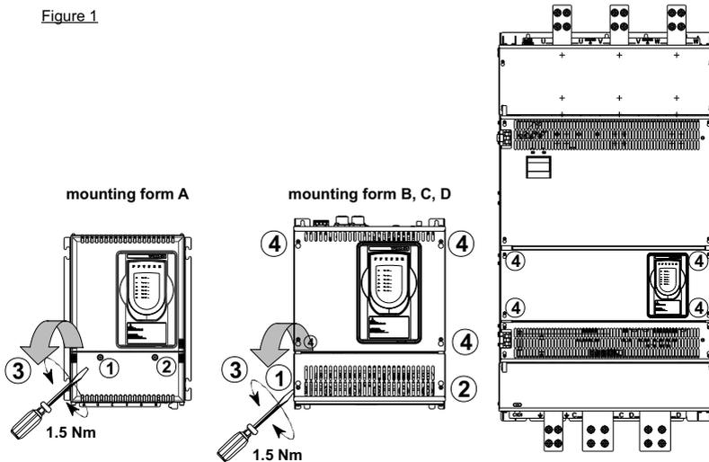
1. The front covers of the devices must be removed to mount the option cards. The devices can be opened without the use of force. Only use the tools specified.
