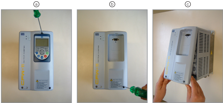
Figure 2: Removal of front cover
