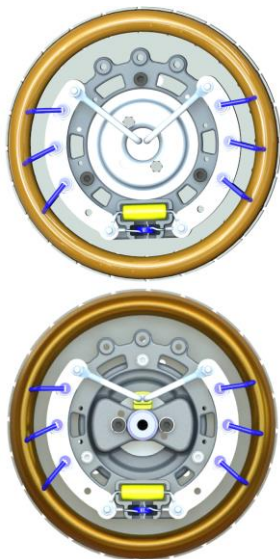
Figure 10.5: Front view of exciter rotor GTA / AG10
