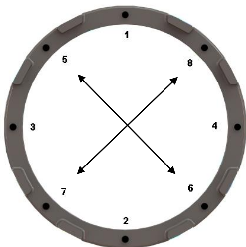
Figure 7.6: Sequence of screws fastening
