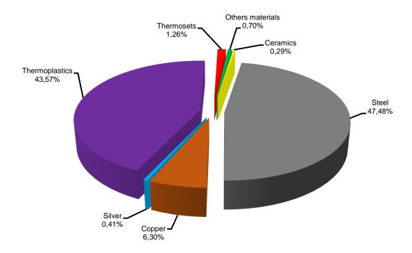
The materials used in the product range and the corresponding weight are disposed below, in *table 1*. The information about the constituent materials is referring to model BU MPW40-3-U010
