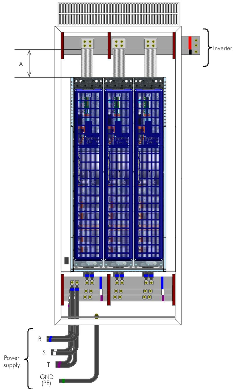
Figure 3.13 - Example of adequate panel installation layout
