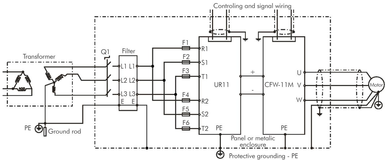
Figure 3.25 - External RFI filter connection for 6 pulse configuration
