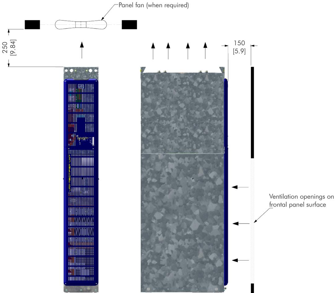
Figure 3.3 - Ventilation clearances in mm [in]
