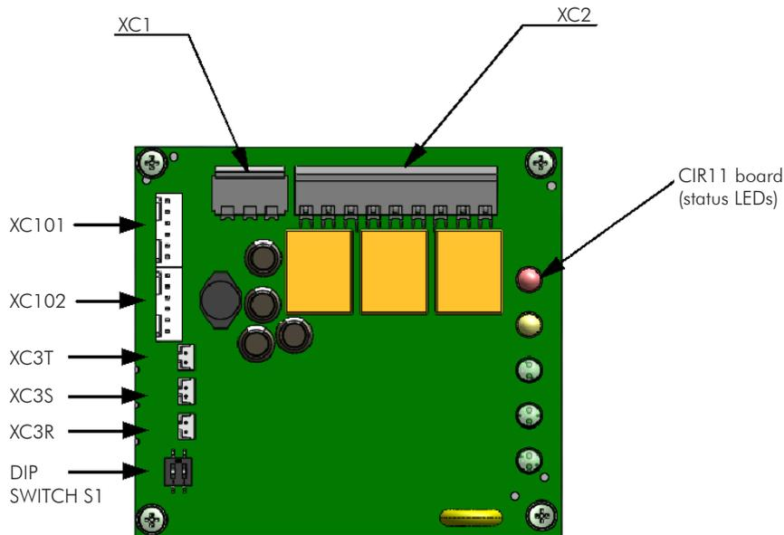
**Figure 3.20 - CIR11 board connection points**
