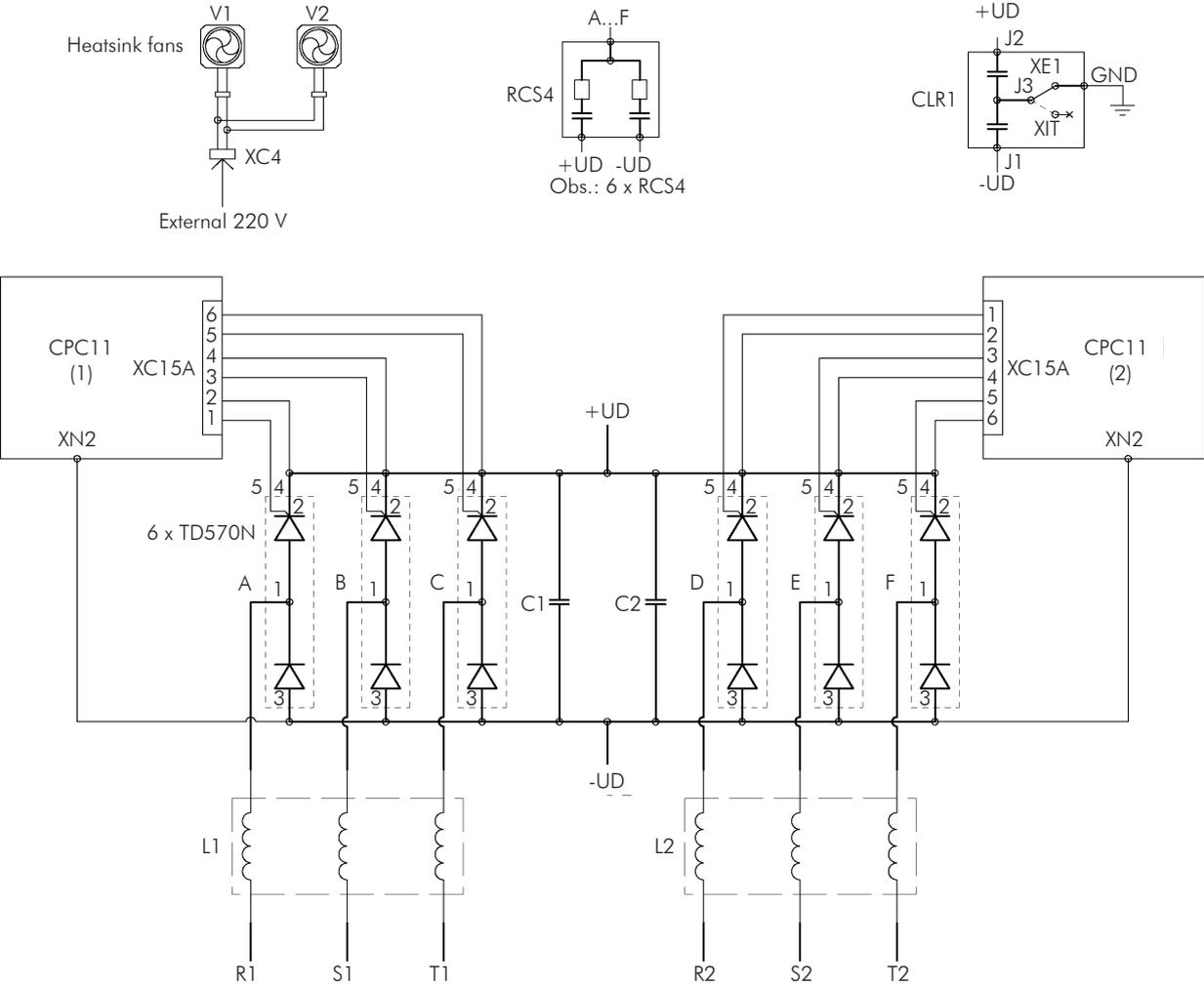
Figure 2.5 - UR11 general internal diagram: power connections
