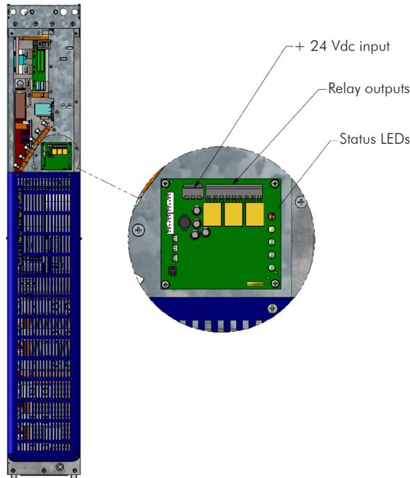
Figure 3.19 - UR11 control cables connection points
