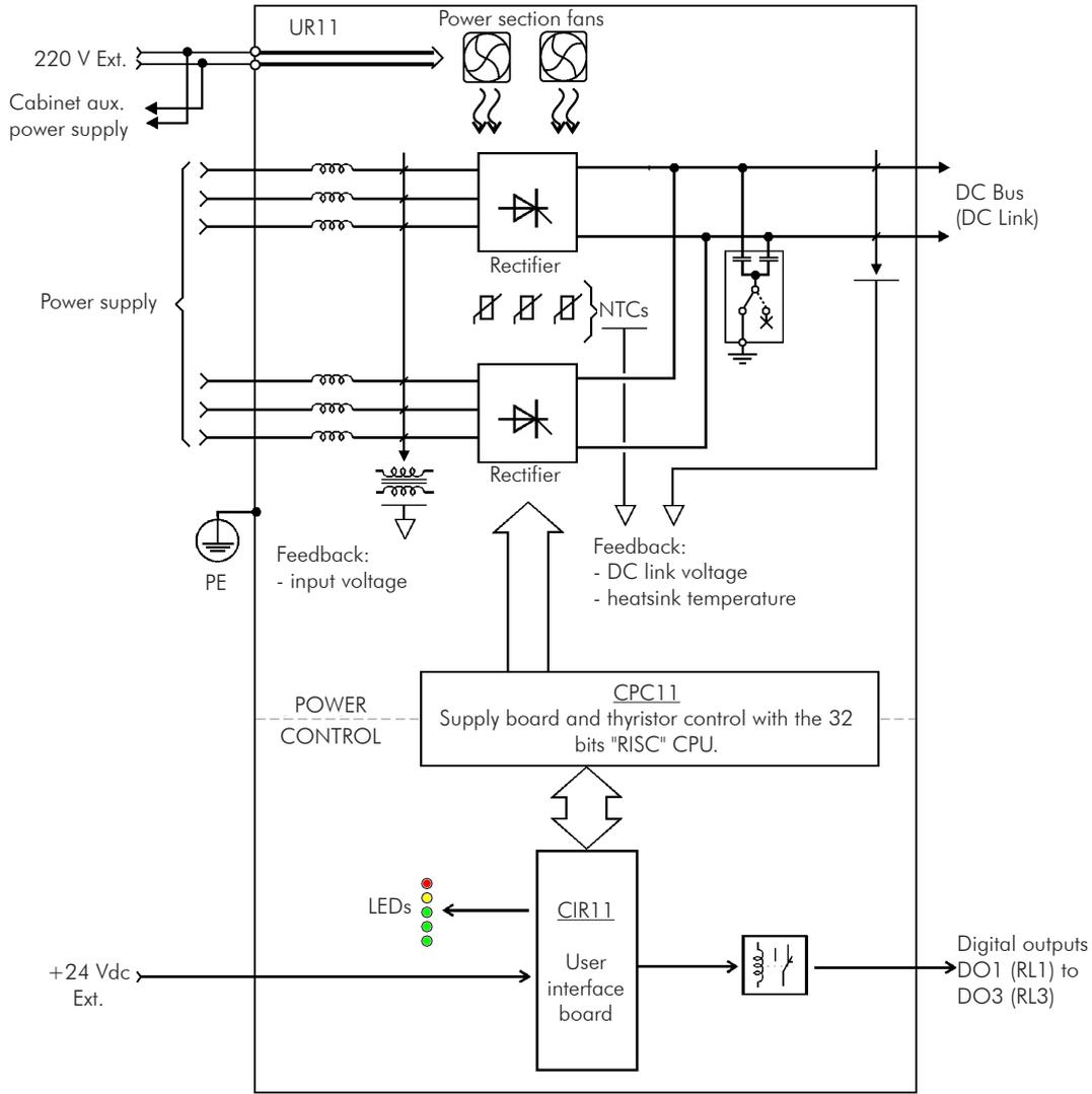
Figure 2.3 - Block diagram for the UR11
