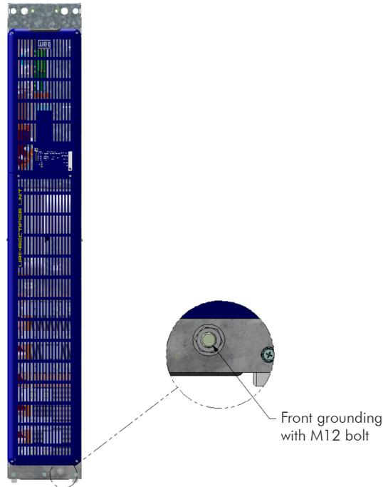
Figure 3.17 - UR11 ground connection point
