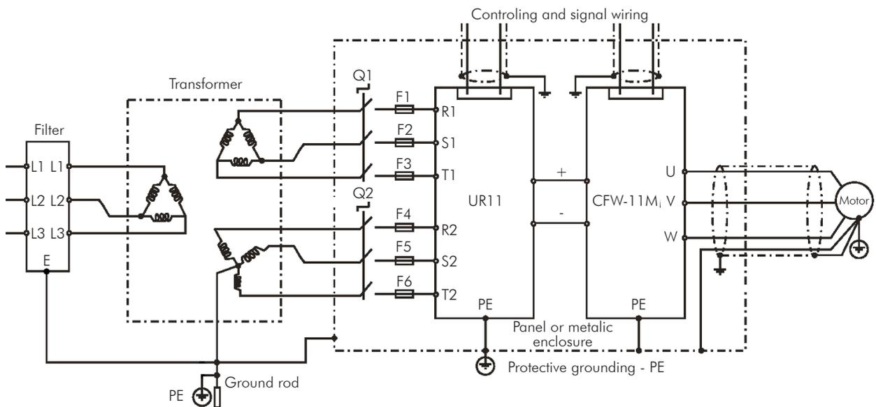
Figure 3.26 - External RFI filter connection for 12 pulse configuration
