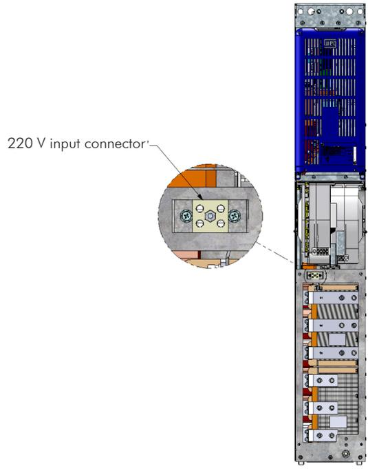
Figure 3.16 - Fans supply terminals: 220 V / 4 A
