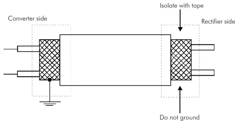
**Figure 3.21** - Cable shield connection
