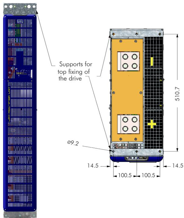
Figure 3.6 - Supports for top fixing (mm [in])
