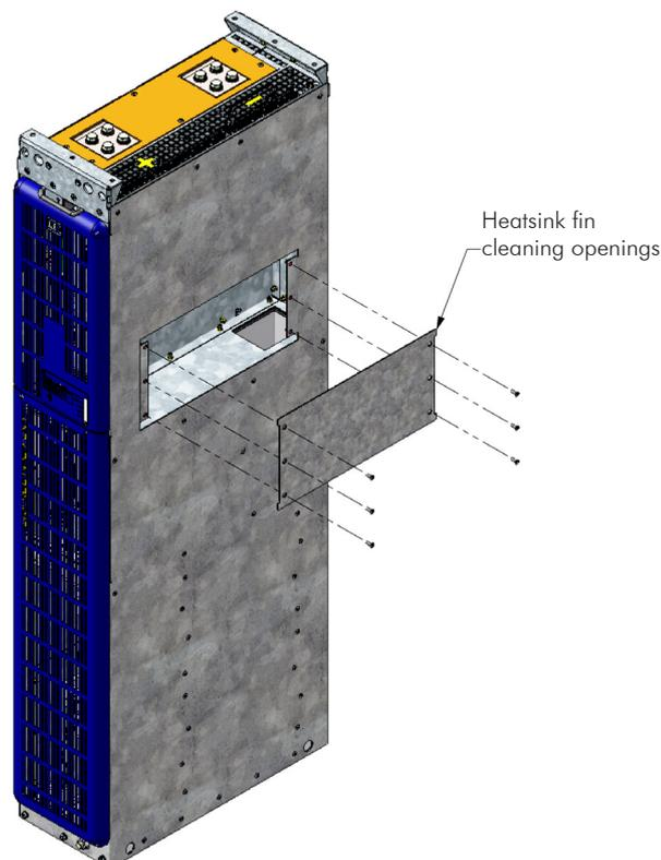
**Figure 5.2** - Cover to get access for inspection/cleaning of the heatsink fins
