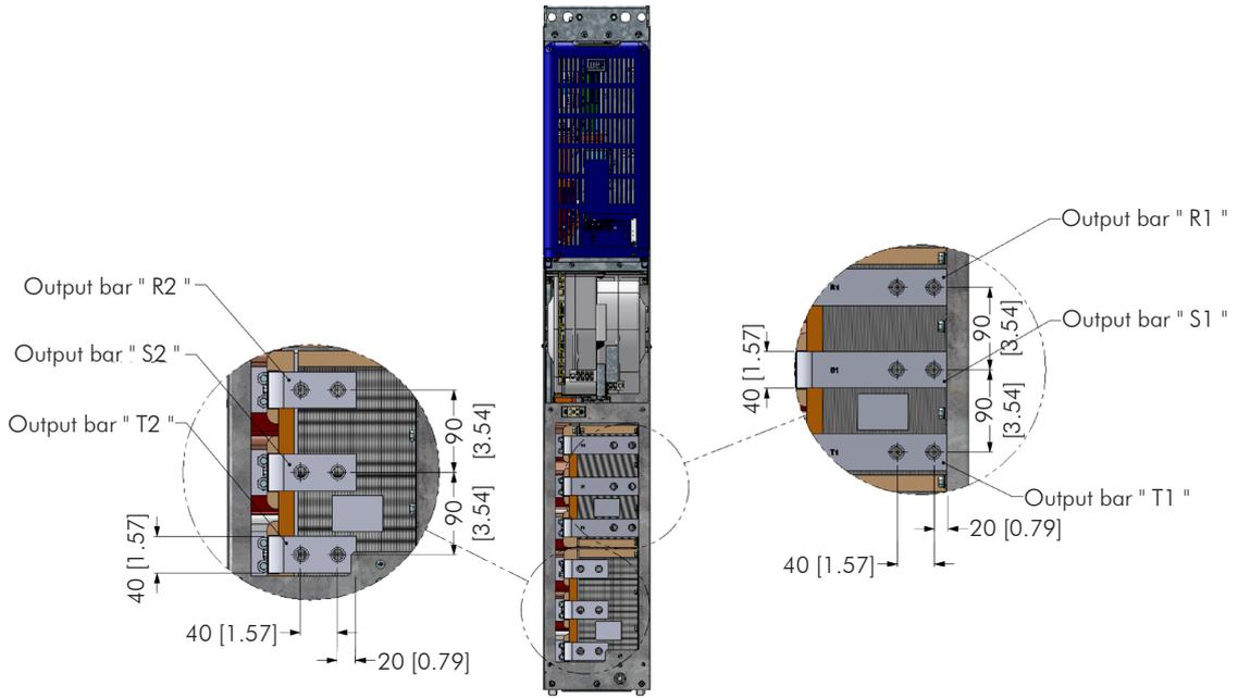
Figure 3.15 - UR11 output bus bar, power supply output connections (mm [in])
