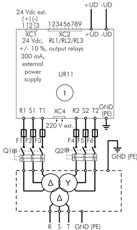
Figure 3.12 - General connection diagram of a 12 pulse rectifier configuration with one UR11 unit
