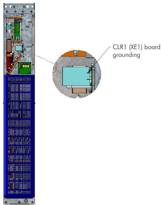
Figure 3.18 - CLR1 board grounding point
