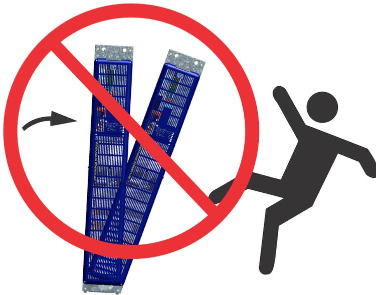
**Figure 2.10** - Do not tilt the rectifier units
