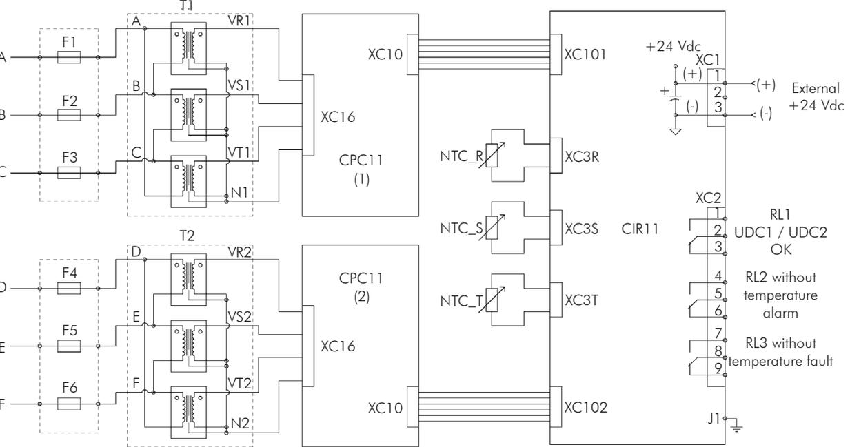
Figure 2.6 - UR11 general internal diagram: control connections
