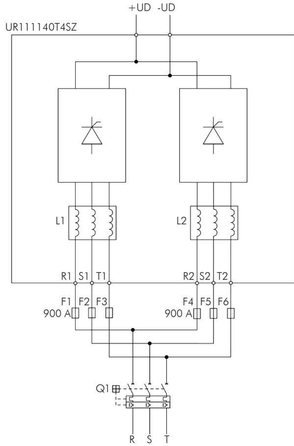
Figure 3.8 - Example of 6 pulse configuration with one rectifier unit
