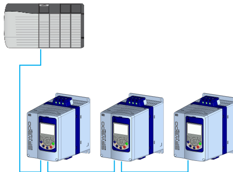
Figure 3.2: Daisy chain topology
