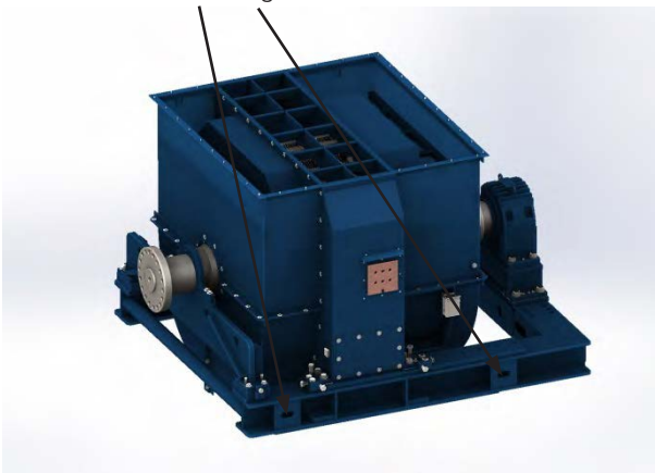
Figure 6-2: Typical Handling of Motor with a Base
