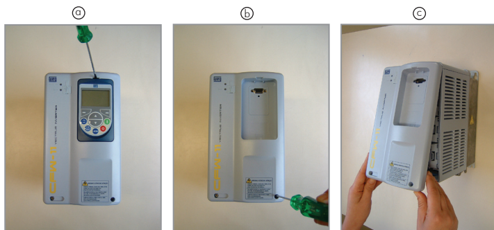
Figure 2: Removal of front cover
