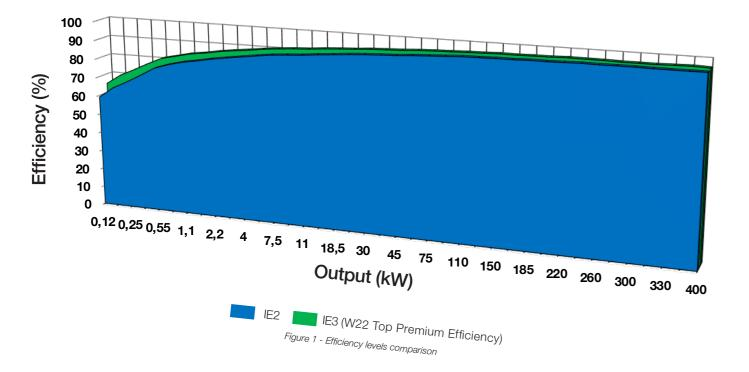
The comparative chart above shows the efficiency comparison between a motor with IE2 efficiency 4-pole machines.
