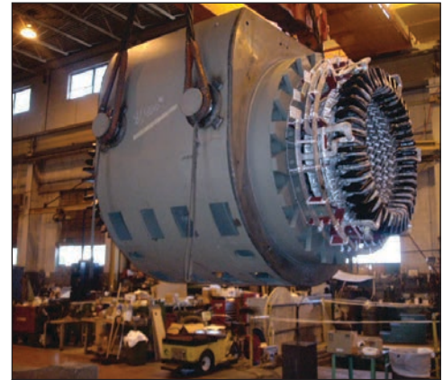
Generator Wound Stator Ready for VPI
