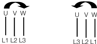
Figure 6.1: Phase Sequence (IEC60034-8)
