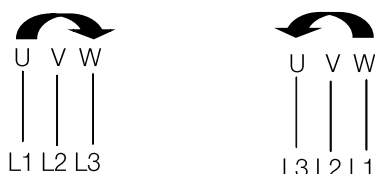
Figure 6.1: Phase Sequence (IEC60034-8)
