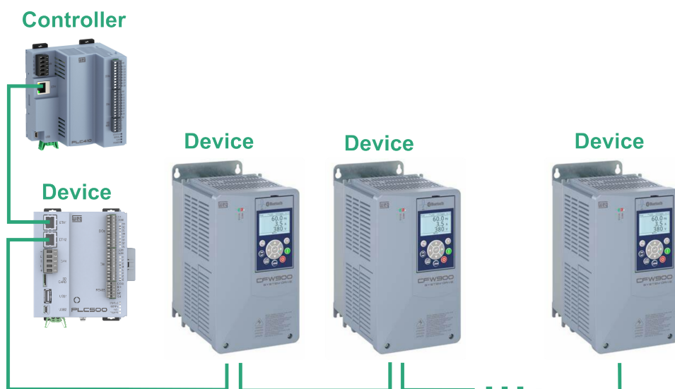
Figura 2.6: Topologia cadeia (daisy-chain) PROFINET.
