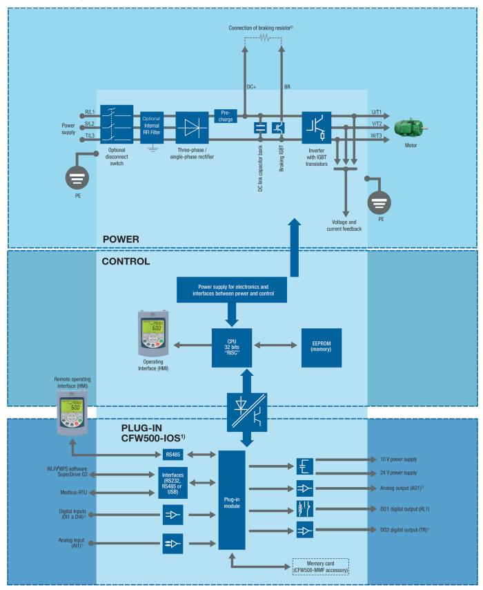
Notes: 1) The number of inputs and outputs (analog and digital), as well as other resources, may vary according to the plug-in module used. For further information, refer to the CFW500 user manual.
