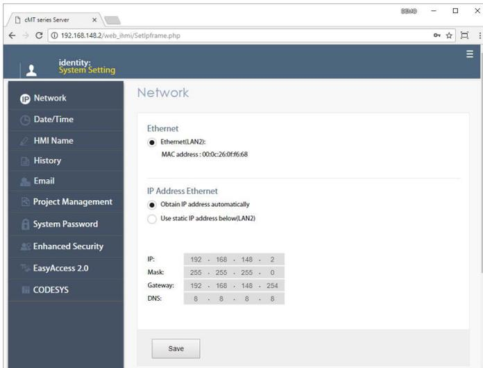
**Step 9:** Go to CODESYS tab and enter your activation code from activation card. Click Activate to activate and enable CODESYS feature.
