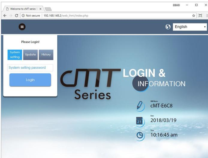
**Step 7:** Enter system password. (Check installation manual for default password).
