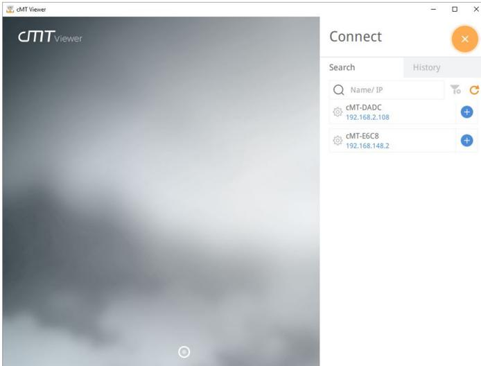
**Step 6:** Open your web browser and enter your HMI IP address. For example, HMI IP address is 192.168.0.211. Enter "http://192.168.0.211" in the address bar and hit enter. If you use cMT Viewer, you can click the setting icon.
