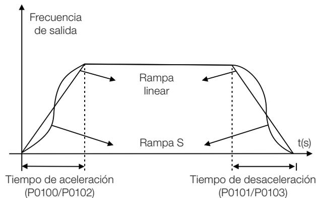
Figura 13.1: Rampa S o Linear
