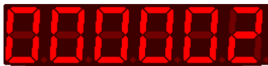
Figure 9.4: Example: last fault indicated on P00036
