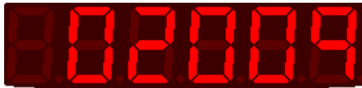
Figure 9.6: Example: year of the last fault (P00038)
