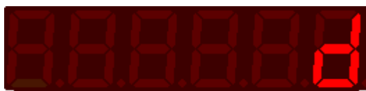
Figure 4.8: HMI screen when downloading the WLP/WPS to the control
