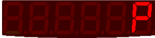
Figure 4.9: HMI screen when the option to load the default factory values is selected
