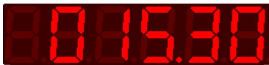
Figure 9.7: Example: hour.min of the last fault (P00039)
