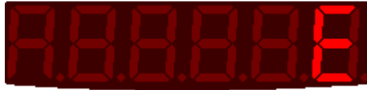
Figure 4.10: HMI screen when you select the option to erase the content of the memory card
