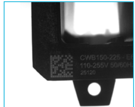
Plastic part with polarized light
