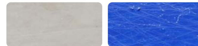
2x zoom in comparison shows damage (microplastics) on silicone-based coating due to cleaning with nylon brushes.
