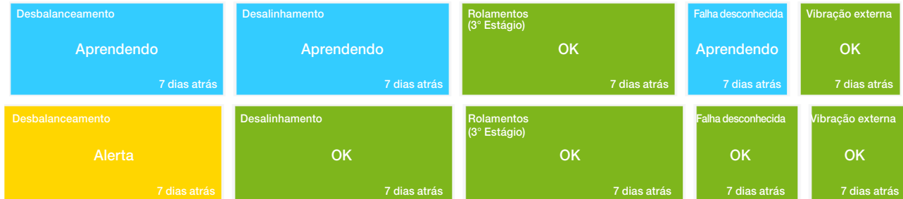
Figure 2.3: View example of the Diagnoses (KPIs) and options: Learning (blue), OK (green), Alert (yellow)
