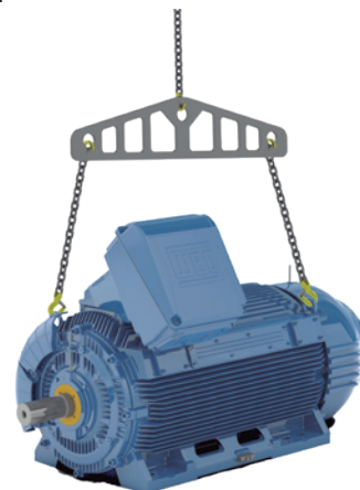
Figure 8 - Lifting with inclined chains.
