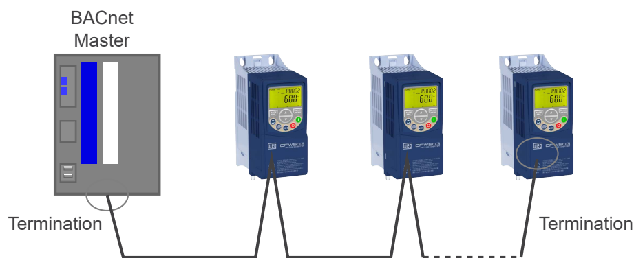
Figure 4.1: BACnet network installation example
