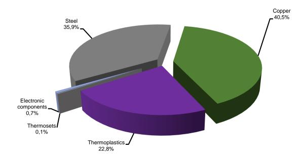
The materials used in the product range and the corresponding weight are disposed below, in *table 1*. The information about the constituent materials is referring to model RWM840E-3-A4U840.
