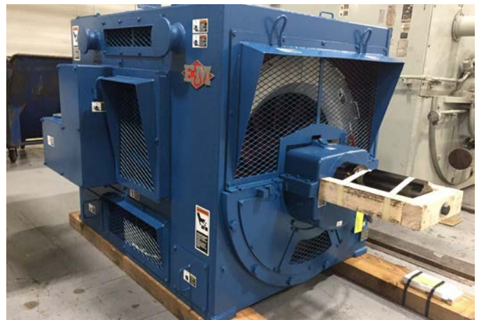
Synchronous Motor Replacement - 1500HP, 12 Poles, 2300V - DPG Enclosure
