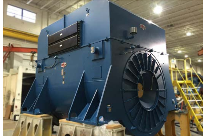
Turbo Generator Replacement - 17647KVA, 2 Poles, 13800V - TEWAC Enclosure
