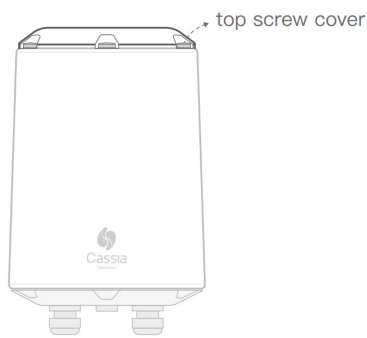
(a) Remova a tampa superior do parafuso
