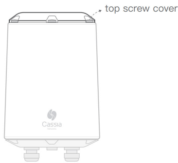
(a) Remove the screw cap
