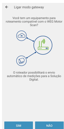
Figure 6.1: Instructions to set up the sensor to gateway mode together with the WEG Motor Scan application
