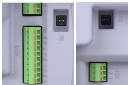
Figure 7 - left: XC10 terminal block (Main input and outputs of the product) and S2 keys (RS 485 resistors), right: XC11 terminal block (Digital output 1, relay contacts) and S1 keys (forced serial communication).
