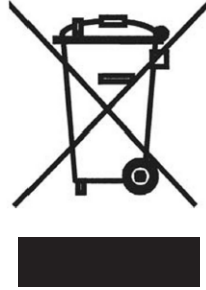
Figure 1 – Indication of selective collection for waste of Electrical and Electronic Equipment (EEE)
