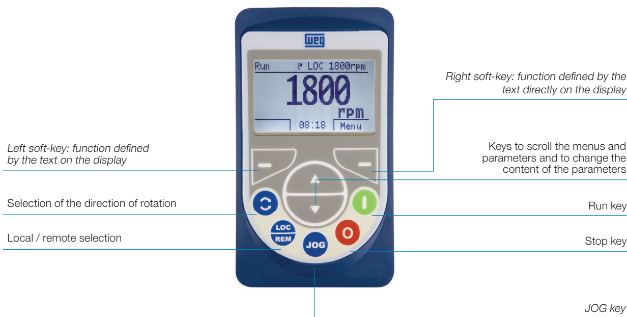
Operating interface (HMI): HMI - 01.
