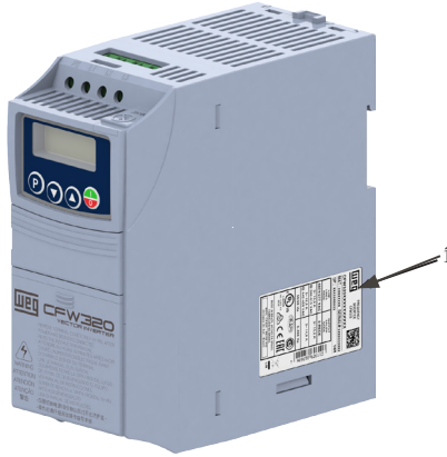
Figure A.2: Location of the nameplate
