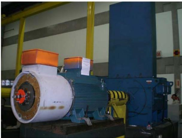
Figure 7 - Doubly fed three-phase induction machine with rotary transformer on laboratory facilities
