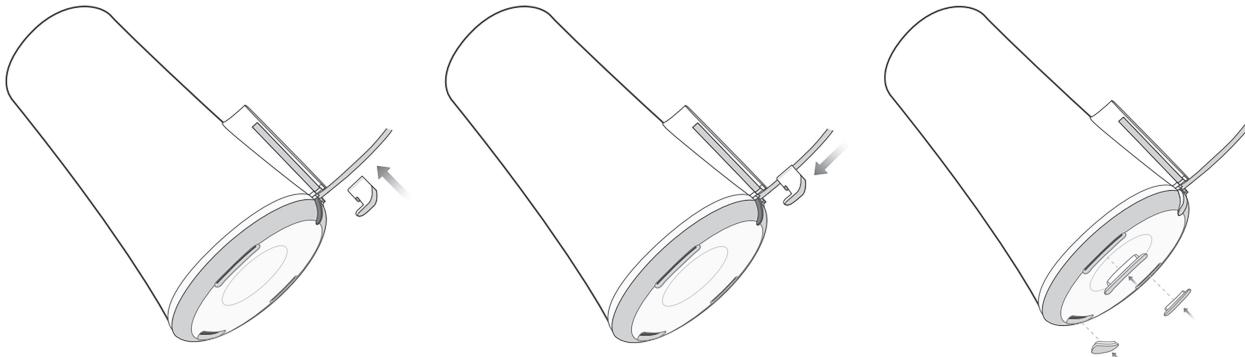
Figure 4.12: Cassia X1000 installing the silicone plugs
