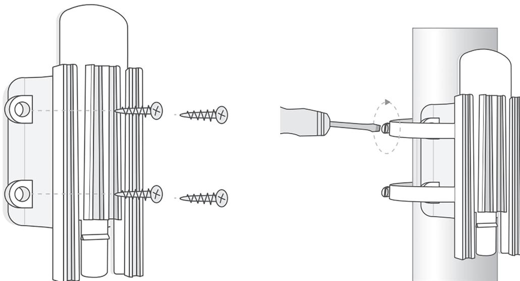
Figure 4.13: Cassia X1000 bracket being installed on wall and pole respectively
