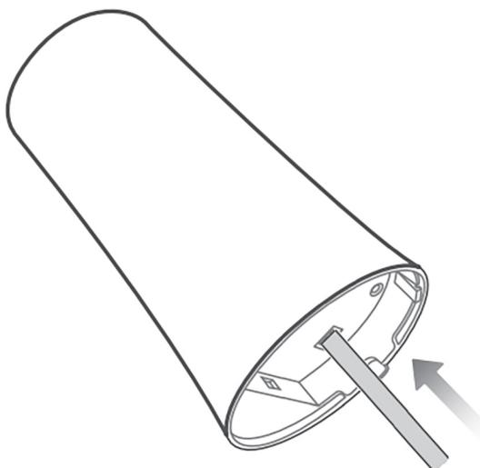
Figure 4.7: Cassia X1000 inserting the ethernet cable
