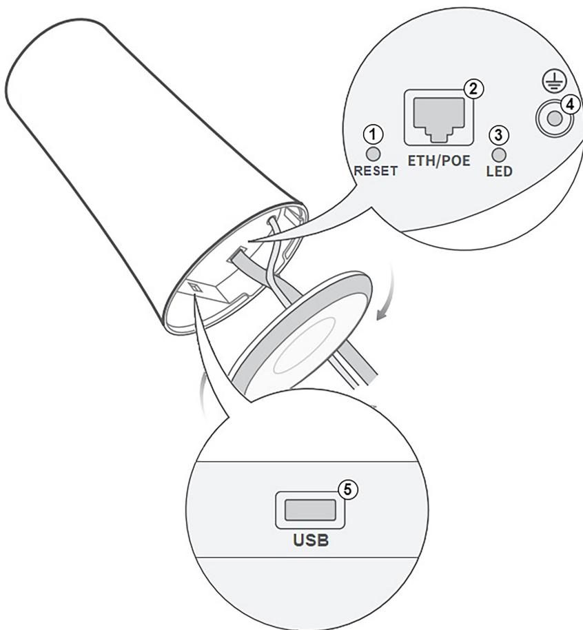
Figure 4.3: Image of the Cassia X1000 gateway with an indication of the connectors and ports
