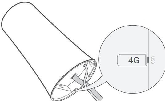
Figure 4.10: Cassia X1000 inserting the 3G/4G dongle
