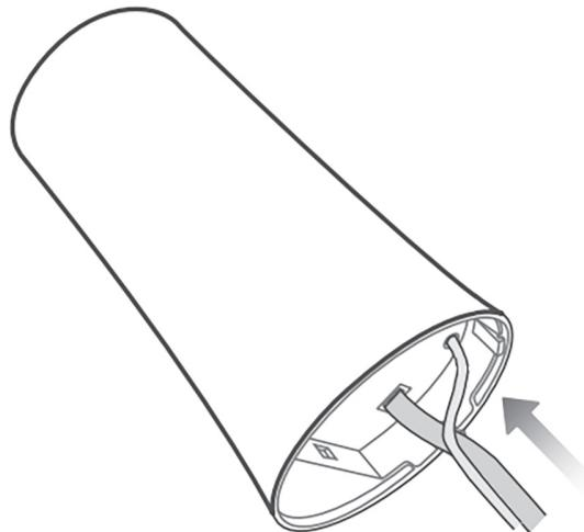
*Figure 4.9: Cassia X1000 inserting the ground cable*
