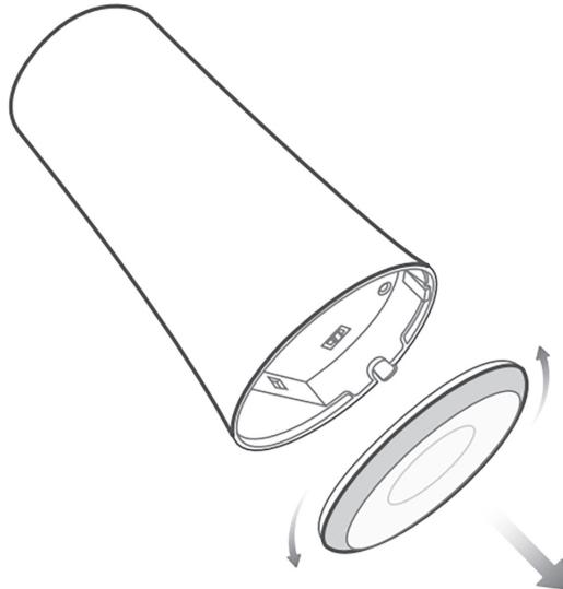
Figure 4.6: Cassia X1000 removing the cover
