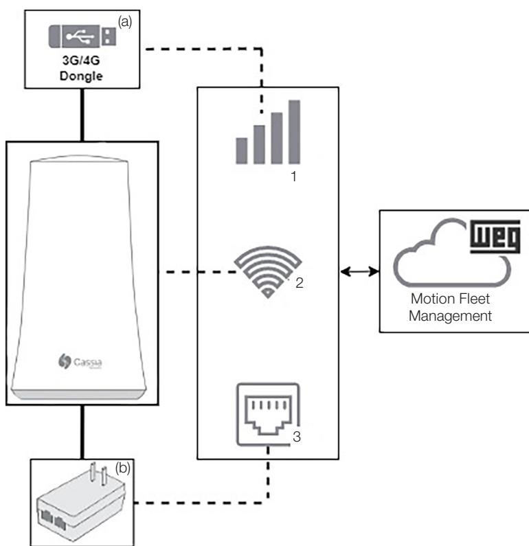
*Figure 4.4: Diagram of internet connection options for Cassia X1000 gateway*
