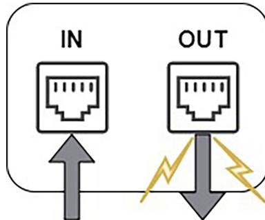
*Figure 4.8: Illustrative image of the RJ45 connectors of the charger included in the Cassia X1000 product*
