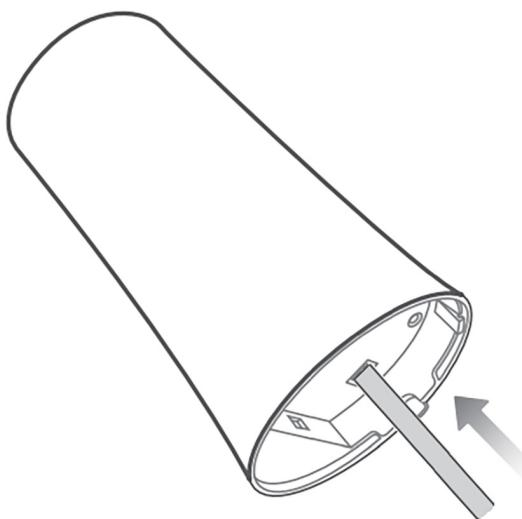
Figura 4.7: Cassia X1000 insertando cable ethernet
