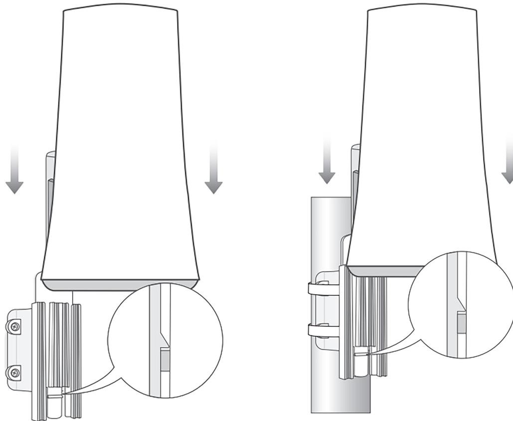
Figure 4.14: Cassia X1000 being fitted to wall and pole bracket respectively
