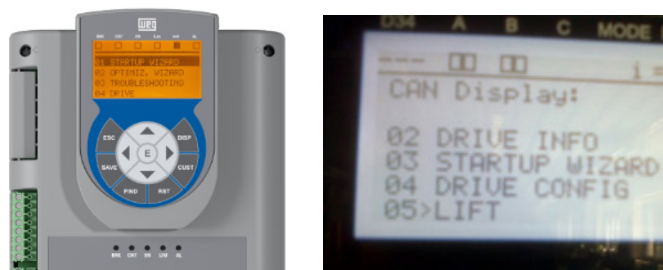
Figure 4: Optional and standard display (Left) and Lift Controller display (Right)
