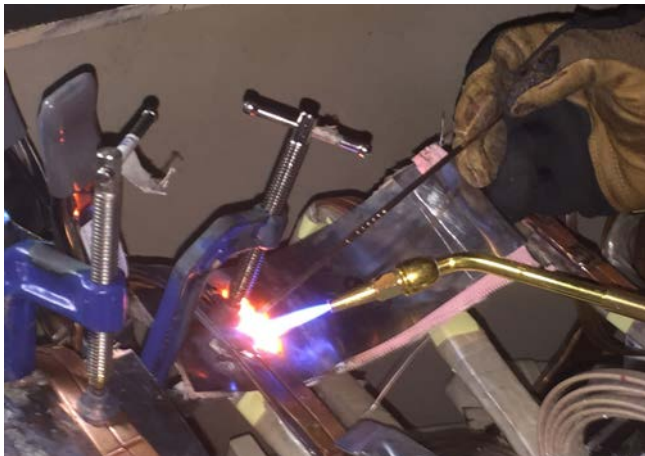
Major winding repairs completed at site by WEG EM technicians
